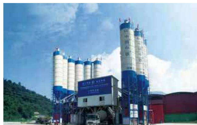
磨万铁路2HZS120V(高铁工程站) 2HZS120V(engineering plant for high-speed railway ) for China-Laos railway construction
