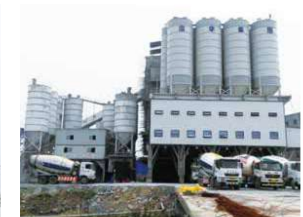
南京海华5HZS270V (顶置环保站) 5HZS270V (bottom-mounted environmental-care mixing plant) in Nanjing Haihua
